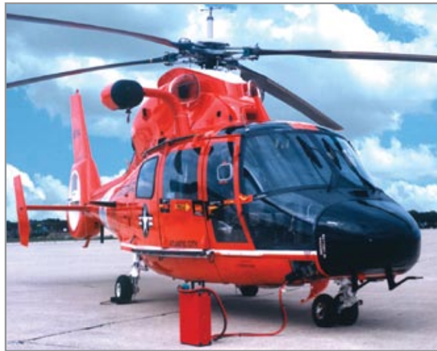
Figure 3.11.4 Starting aircraft with TI1000 GPU-24
