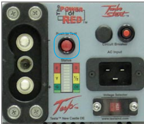
Figure 2.11.1 - “Push to Test” button location (outlined in blue)
