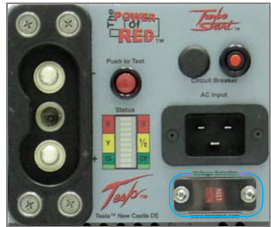
Figure 2.10.1 Input Voltage Selector Switch (outlined in blue)
