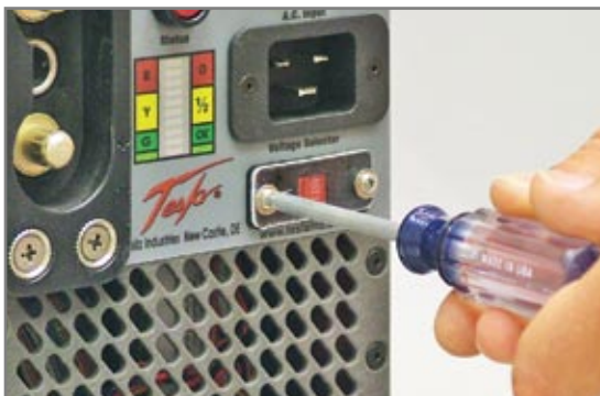
Figure 2.10.2 - Unscrew Protective Cover
