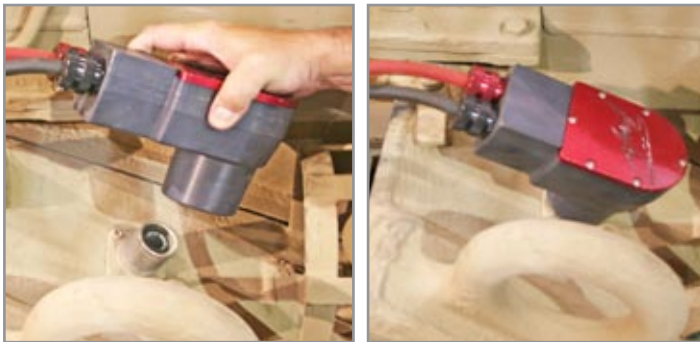
Figure 3.11.2 Attaching NATO DC Power Cable to vehicle
