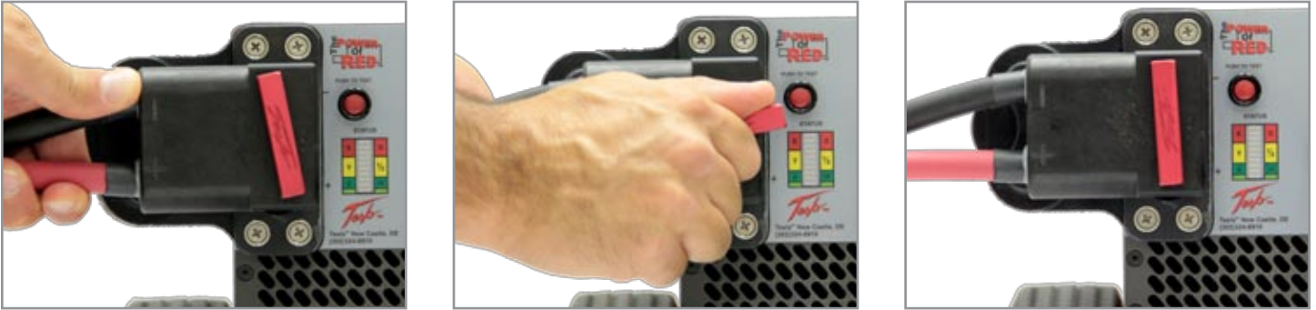
Figure 3.11.1 Attaching DC Power Cable to GPU
