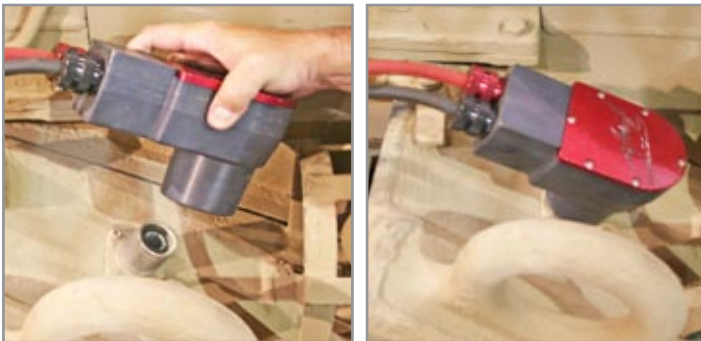
Figure 3.11.2 Attaching NATO DC Power Cable to vehicle
