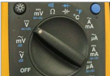
1. Set multimeter to Volts.
