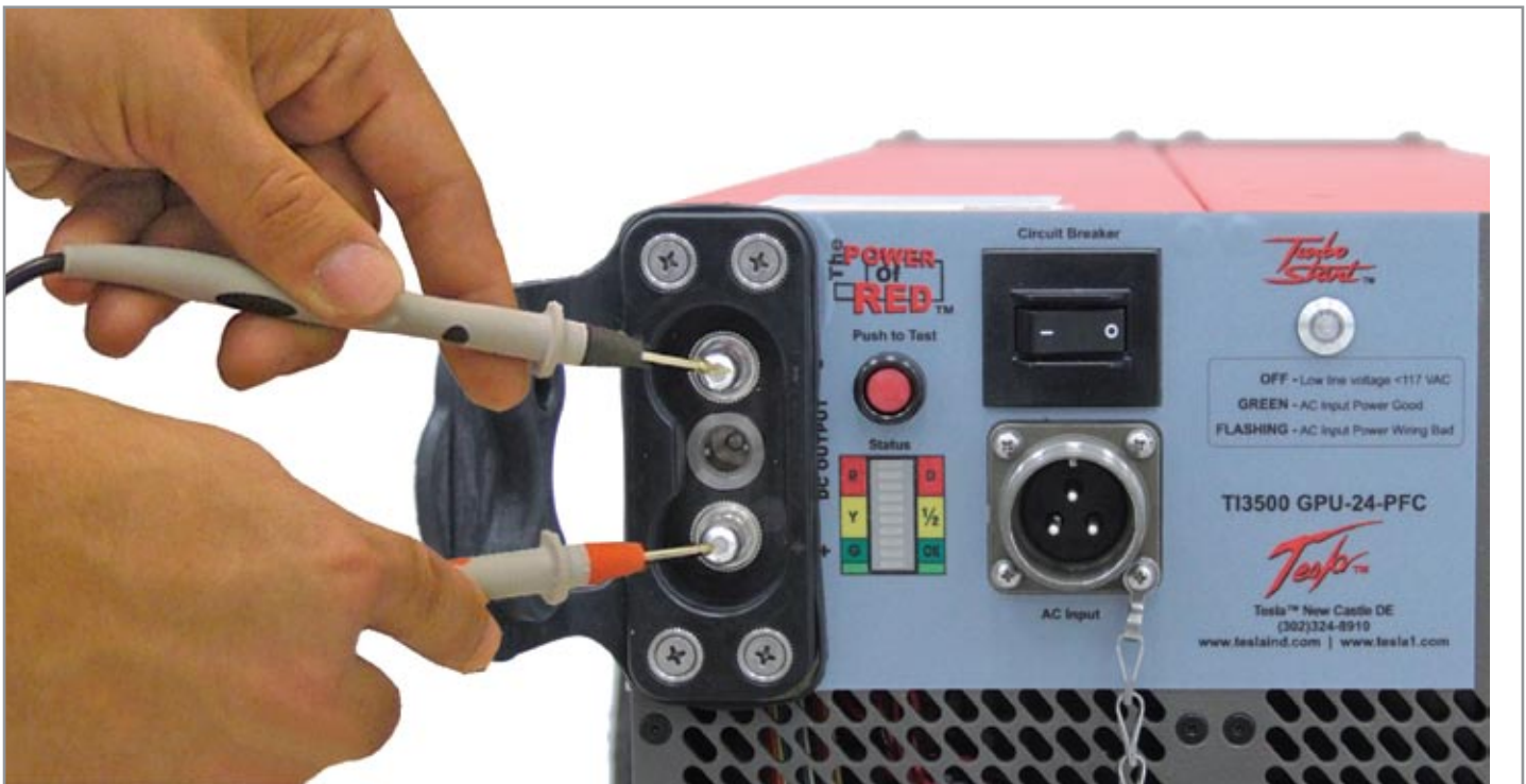
Figure 3.8.2 – Testing DC Receptacle
