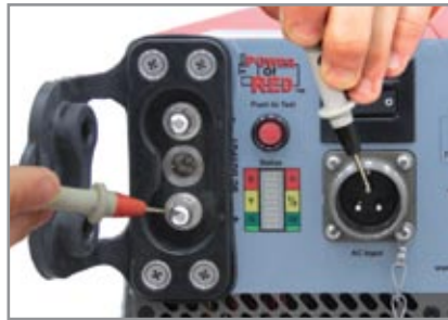
2. Place the negative probe on the ac ground post of the ac input and the positive probe to the dc positive post. Multimeter should read greater than 10 M \Omega .
