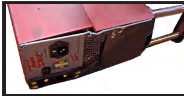
Figure 5-3: Misalignment Case with Bent Face Plate
