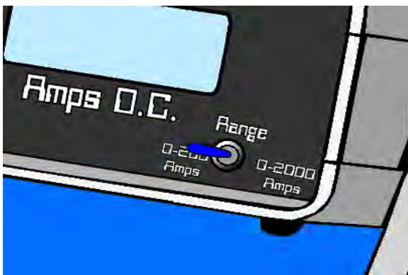
Figure 6-25: DVAM Switched to 0-200 Amps
