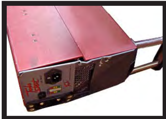
Figure 8-7: Misaligned Case with Bent Face Plate
