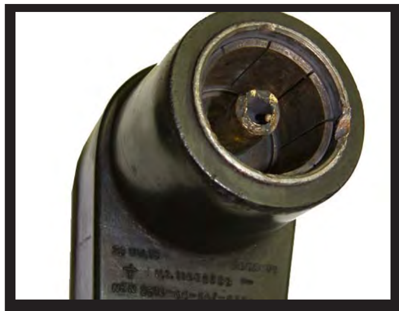
Figure 8-5: Damaged NATO Plug
