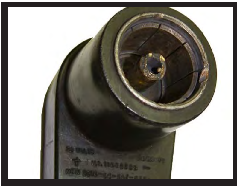
Figure 5-5: Damaged NATO Plug
