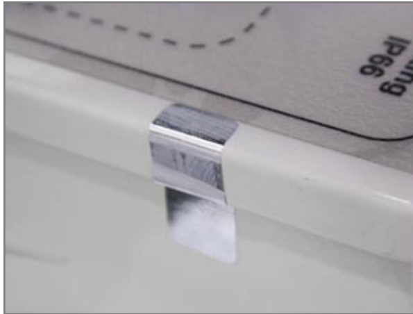
Figure 4.1.1 - Warranty Void stickers are on the sides of the unit
