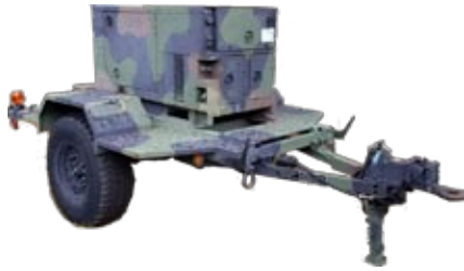
5K / 10K Generator
